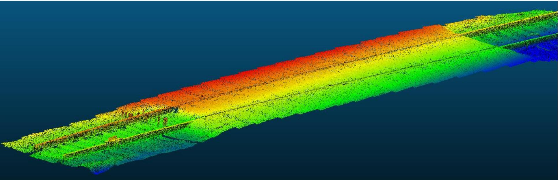
Using the 3D point cloud, crossing roughness may be quantified as depth and area of cracks, area and volume of bumps or pot-holes, or other formulations. An example displaying surface curvature gradient is illustrated below. **Blue** areas are relatively flat as compared to **Red** areas in this visualization.
