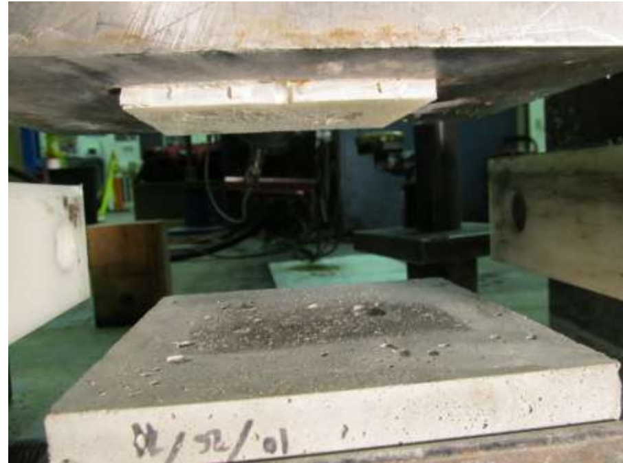
Pad material confined to cavity in loading head
