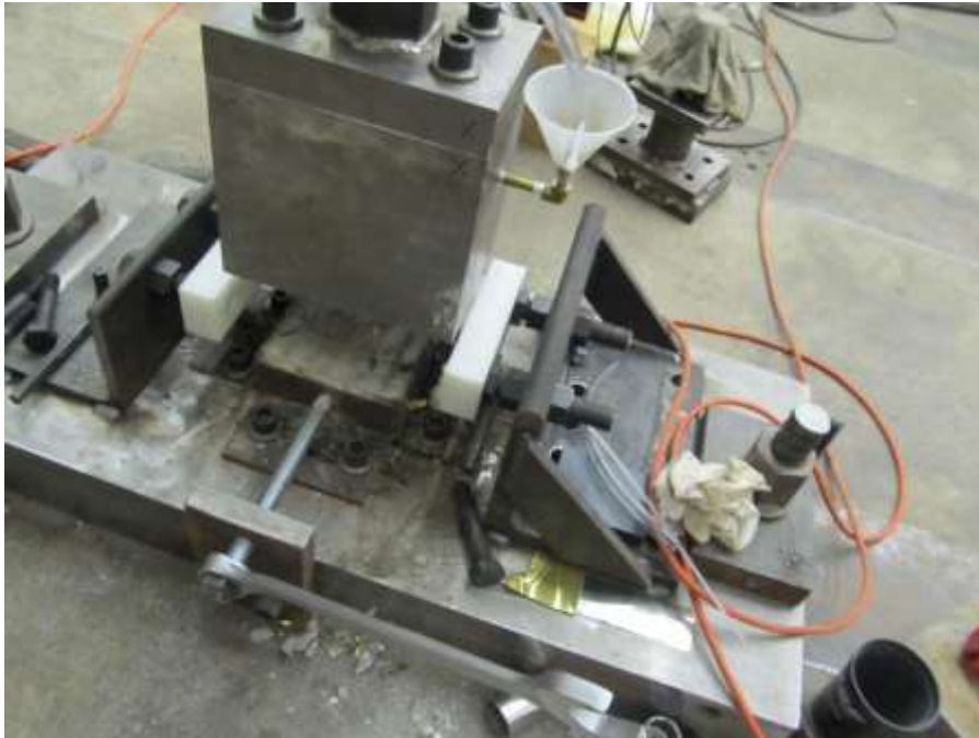
Loading head and concrete specimen fixed to strong floor
