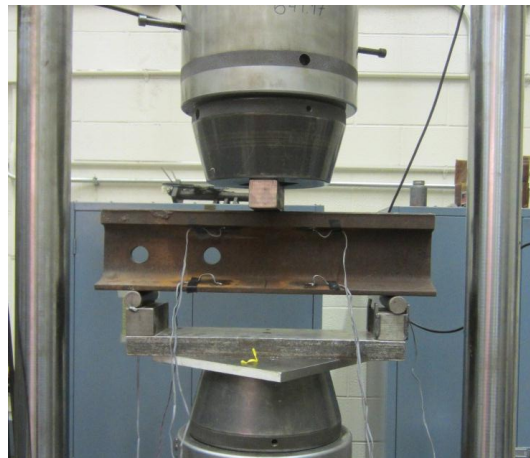
Figure 1: Simply supported instrumented segment of rail in 3-point bending
