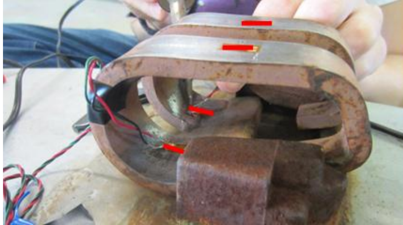
Figure 3: Gauge side fastener showing placement of strain gauges (in red).
